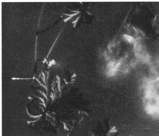
Figure 8 Sheaving structures in polysulphone film cast from dichloromethane/carbon tetrachloride. Crossed polaroids plus tint plate ( \times 700 ).
